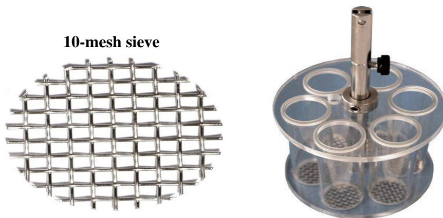
Fig 2.3: Parts of disintegration test machine
